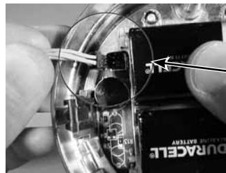
Wire connector being inserted into the receptacle on the keypad circuit board.
